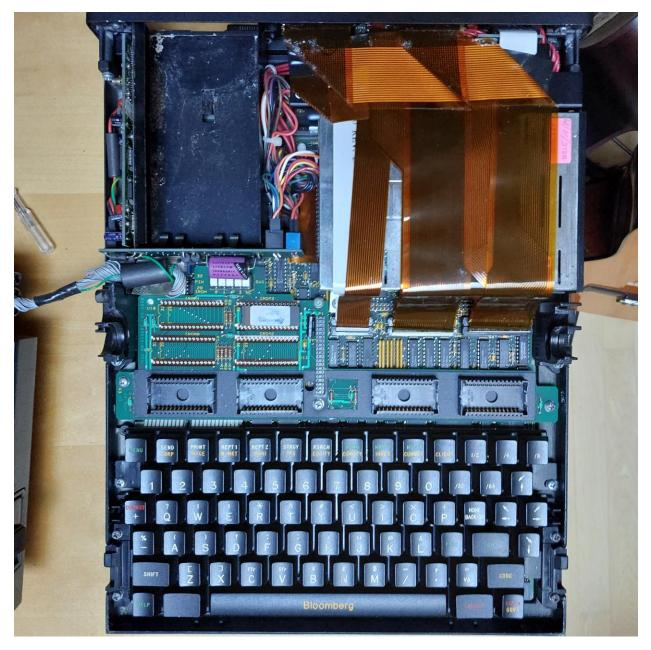
The keyboard cables were disconnected from the motherboard and 22 wires were soldered from the keyboard to the Teensy 4.1 I/O pins per the following table. Note that Teensy I/O 13 was skipped because it is connected to the onboard LED. Teensy I/O 15 was not working correctly so the wire was moved to I/O 24. A Teensy 4.1 was used (because it was available) but any other Teensy could be used with no code changes.
