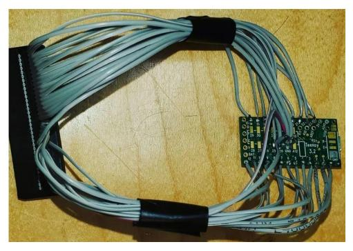
The table below shows how the ribbon cable was wired to the Teensy 3.2.
