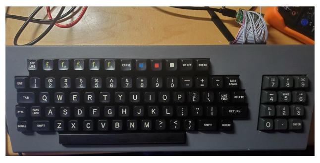
Note the odd key layout for the bracket keys, the lack of a Num Lock key, and several keys that do not exist on a modern keyboard. These odd keys are not implemented because they don't have any USB HID codes.
