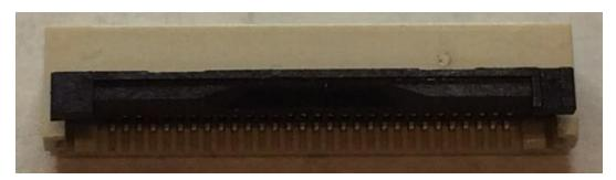
The FPC cable had nubs on each side that were trimmed off with scissors so it would fit in a generic 30 pin 0.5mm pitch connector.
