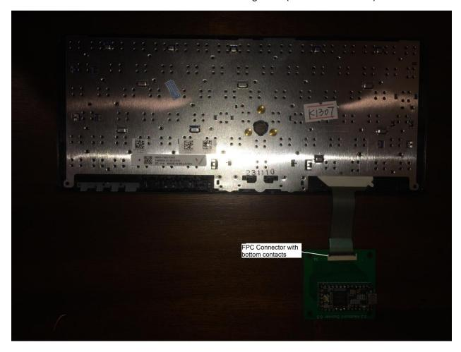
The Teensy will sit underneath the keyboard when the FPC cable is looped back as shown.
