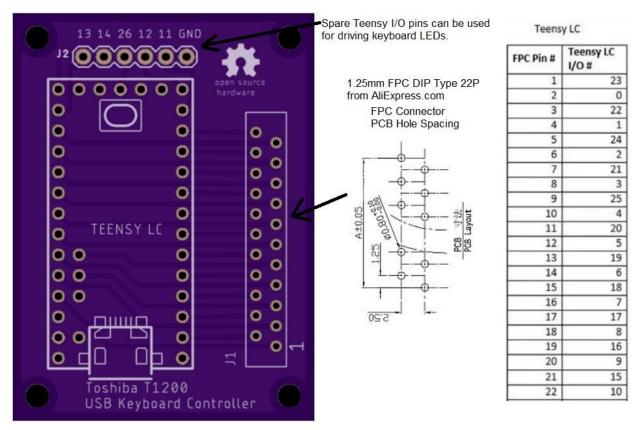
The Eagle board file "T1200.brd" can be fabricated directly by OSH Park. The zipped Gerber file "T1200\_2020-04-27.zip" is formatted for fabrication by JLCPCB.
