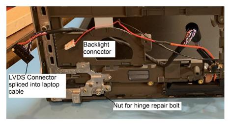
The Toshiba laptop hinge is prone to failure over time. The pictures below show the good right hinge and broken left hinge. A hole was drilled so that a bolt and washer could repair the hinge.
