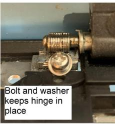
The left speaker had to be milled out with a Dremel to make space for the hinge repair screw.
