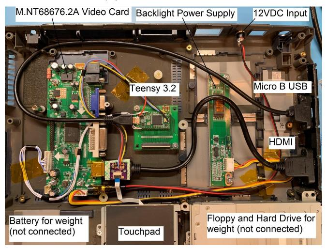
A small board was designed for the touchpad FPC cable with a connector so that the signals can be jumpered to the Teensy per the table below. The FPC cable flips the signals so the pin numbers are the same on both ends of the cable.
