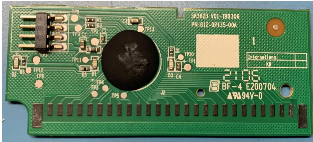
Original keyboard controller "blob top" IC
