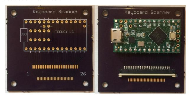
All of the signals for the Teensy LC are routed on one side of my board so I designed the other side for a Teensy 3.2 with 34 I/O signals and an FPC connector with a 1 mm or 0.8 mm pitch. If you need all 34 pins, you must unsolder the LED on the Teensy 3.2 to free it up for use by the keyboard.
