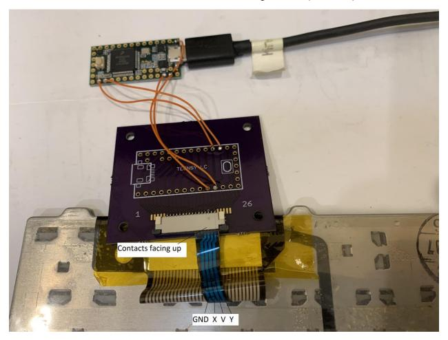
This also shows how the keyboard FPC cable and the pointing stick FPC cable have been taken out of the solderless connector used on the motherboard. I had to pull off the extra thick plastic backing on both FPC cables. The pointing stick cable had its sides trimmed with scissors and then two pieces of "stick-up" paper were attached to bring the thickness back to the normal 0.3mm so a generic connector could be used.
