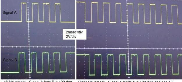
Left Movement - Signal A lags B by 90 deg and has 8 clock edges.
