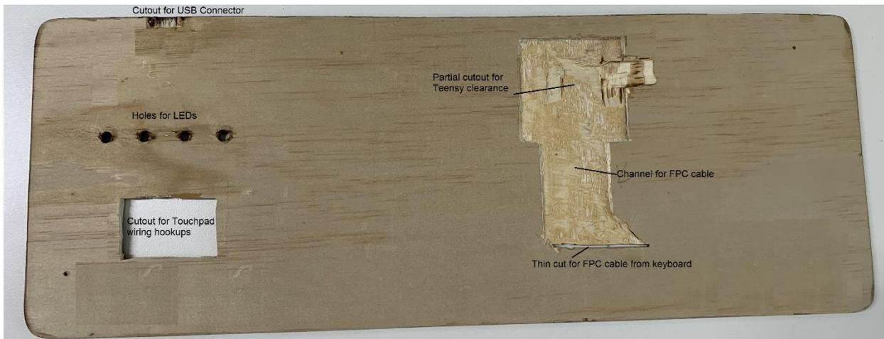
Bottom and middle plywood sheets have been glued together in the picture below. The Teensy Keyboard Scanner board is screwed down and the Adafruit 1833 USB micro B breakout board is wired to a USB micro plug that goes into the Teensy connector. This connector and the reset push button are the high points on the Teensy. Wood was removed from the top plywood at these locations to eliminate any clearance issues. All wires are held in their channels with Kapton tape.
