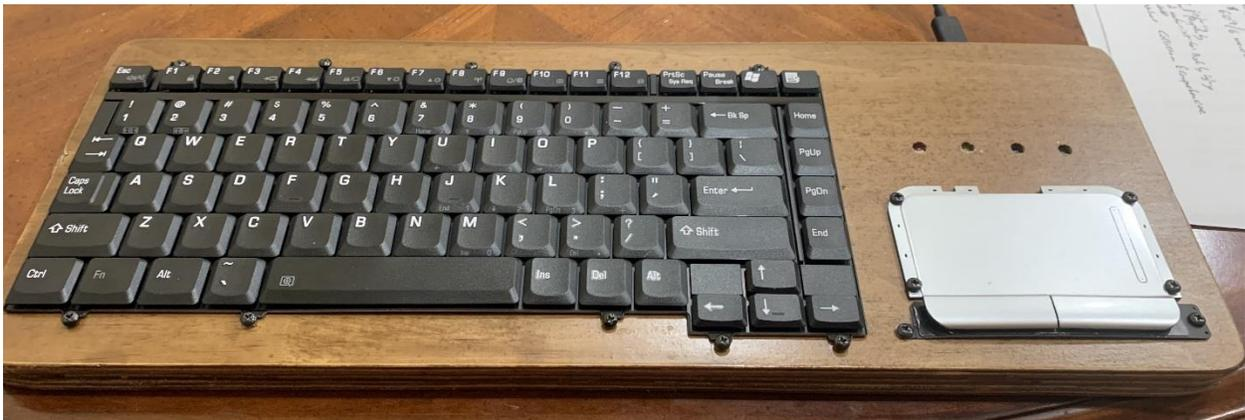
The overall dimensions are  $16 \frac{5}{8}'' \times 6 \frac{1}{8}'' \times \frac{11}{16}''$ . I initially used plastic washers on all the keyboard screws but found they were not needed. Also, washers raise the screw heads up higher, causing them to be felt when pushing the nearby key.
