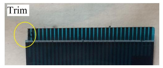
The Dell Latitude D630 keyboard needed the most modifications. It had a solder-less connector on the end of the FPC cable that was easily removed. Then I pulled off the extra thick plastic backing that was glued on the end of the cable and cut a notch on the side to align the contacts. To bring the thickness back to normal, I glued 2 pieces of paper to the end of the cable (see below).
