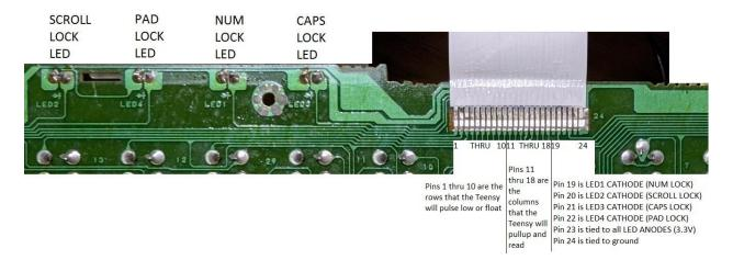
The FPC connector has a pin 1 marking on it but it may not coincide with the pin 1 position on the circuit board. Rotate the connector 180 degrees if necessary to make the exposed metal traces on the FPC cable coincide with the metal contacts inside the connector (see below).
