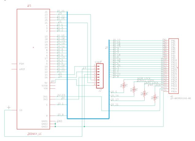
The unused I/O's, plus power and ground are brought to solder pads at J2 for future use. I/O 13 can drive up to 5ma. It currently drives the LED on the Teensy with 3ma.
