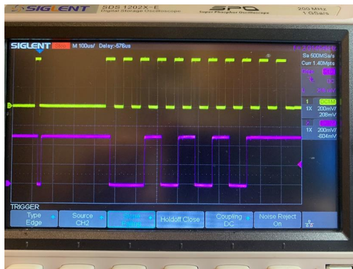
Clock and Data signals on Motorola 4824402E pins
