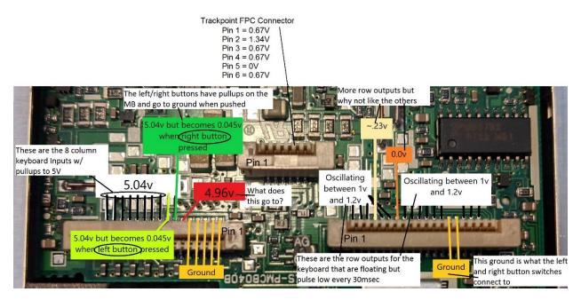
16 pin FPC connector - The first 5 FPC pins are strapped to ground to identify the keyboard as a US language configuration. Later testing showed that pin 6 is for the Fn key. The right and left trackpoint buttons on pins 7 and 8 are pulled up to 5 volts and go to ground when the buttons are pressed. Pins 9 thru 16 are the 8 columns for the key matrix and are pulled up to 5 volts.
