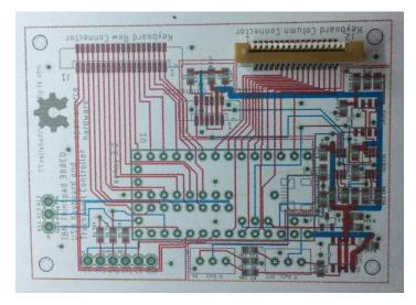
With the paper layout showing no problems, the <u>Eagle board file</u> was sent to OSH Park for fabrication. 3 boards cost \$27 to fabricate. The board is 50mm x 70mm and uses the default settings.
