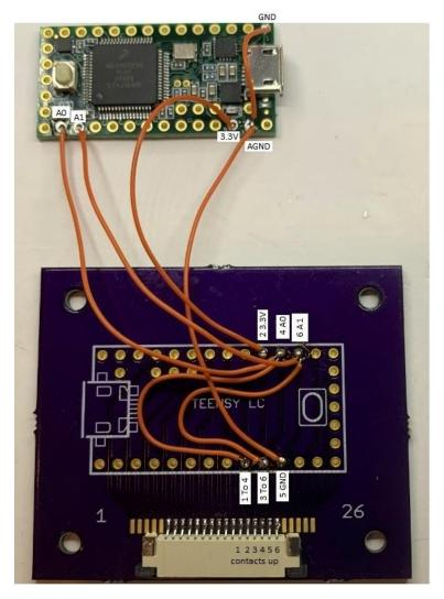
FPC Pin 2 goes to Teensy 3.3 volts. Pin 5 goes to Teensy ground. Pins 3 and 6 go to Teensy ADC A1 and pins 1 and 4 to Teensy ADC A0.
