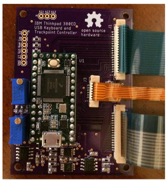
I designed the layout so that 2x7 right-angle <u>header pins</u> can be used for the surface mount pads on the Teensy backside instead of flying leads.
