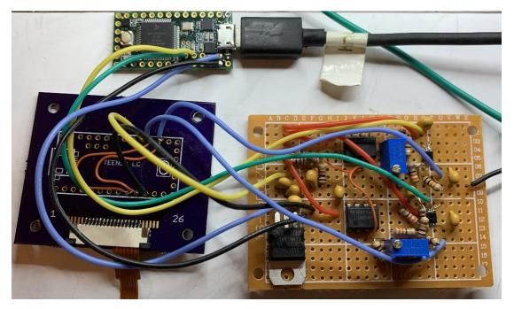
Both potentiometers smoothly adjusted the instrumentation amps to output 1 volt with the trackpoint at rest. Pushing the trackpoint hard in each direction gave these voltages out of each AD8236.
