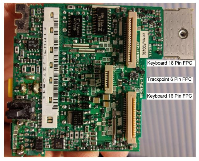
The 3 FPC cables were installed and the daughterboard plugged into the motherboard in order to measure the voltages on the connector pins. Note that the first 5 FPC traces on the 16 pin cable don't go to the keyboard. Pin 1 is open and pins 2 thru 5 are tied together as shown below.
