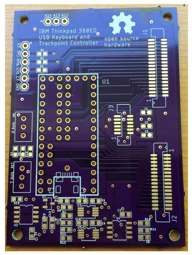
I used standard tin-lead solder paste, applied with a syringe and toothpick, then re-flowed with a <u>converted toaster oven</u>. I had to clear a few solder bridges where I applied too much paste. The old saying "the bigger the blob, the better the job" does not apply with surface mount devices.
