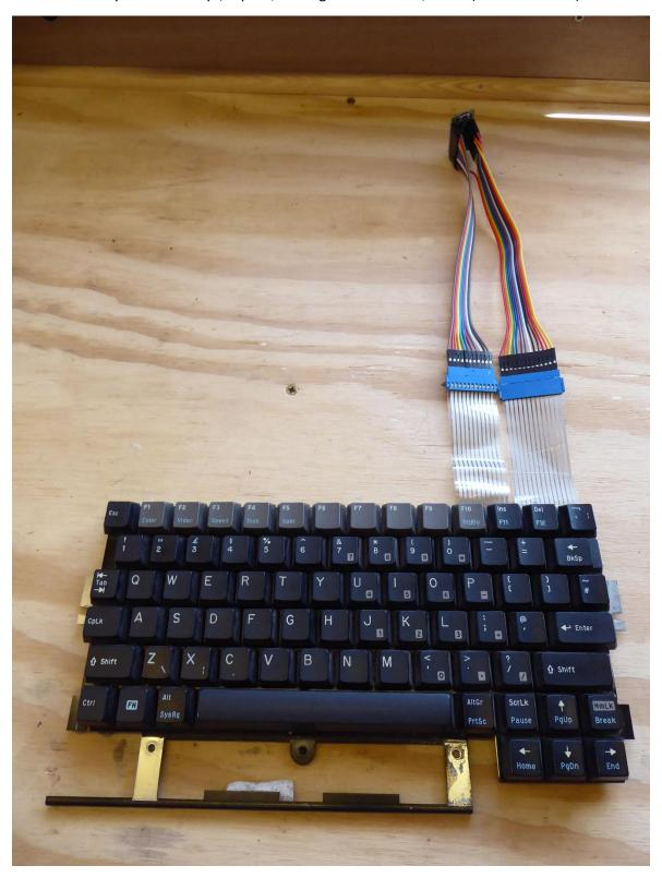
Running the matrix decoder code provided the 11 x 13 key matrix which was converted to the Teensy LC I/O pins, as shown below.
