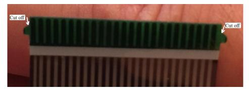
If the FPC traces don't line up with the connector pins, use an X-ACTO knife to trim along the side of the cable.
