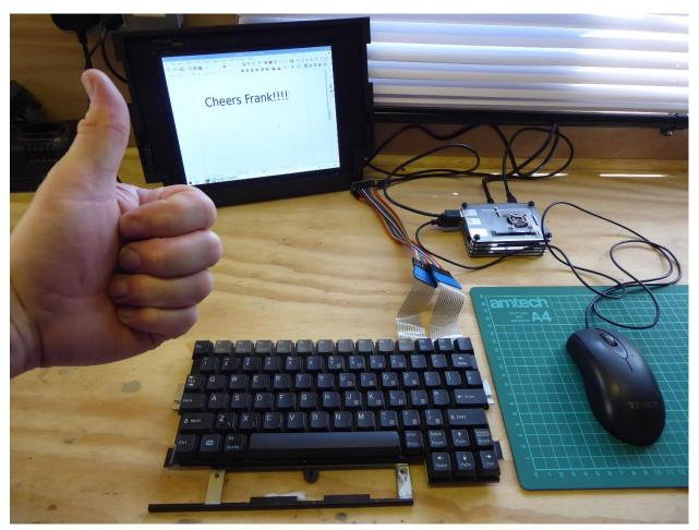
Here is the GRiD keyboard & Teensy connected to a Raspberry Pi that is driving the GRiD display.
