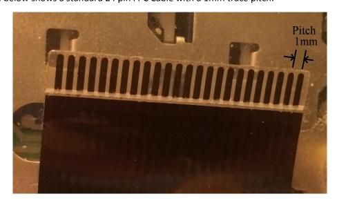
Some FPC cables need to be modified to fit in a generic connector. Locking nubs on the side of the cable are easy to remove with wire cutters.
