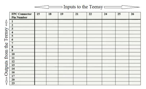
The orientation of the keyboard matrix is just my personal preference. You can swap the rows/columns and inputs/outputs if you want. Swapping pins may be necessary if you have a rare laptop keyboard that has diodes on its switches.
