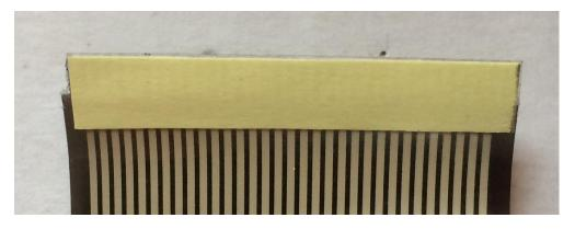
I designed a circuit board using Eagle for the Teensy LC that routes its 26 I/O pins to 26 surface mount pads for an FPC connector with a 1mm pitch or 0.8mm pitch. A 24, 25, or 26 pin FPC connector can be soldered to this board based on your needs. I avoided using the 27th Teensy LC output because it's connected to an LED and 27 pin FPC connectors are rare.
