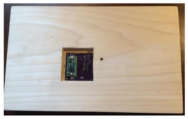
You'll have to drill a hole into the cavity for the USB cable and glue rubber feet on the backside.
