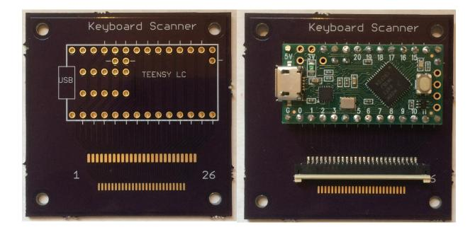
All of the signals for the Teensy LC are routed on one side of my board so I designed the other side for a Teensy 3.2 with 34 I/O signals and an FPC connector with a 1 mm or 0.8 mm pitch. If you need all 34 pins, you must unsolder the LED on the Teensy 3.2 to free it up for use by the keyboard.
