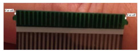
If the FPC traces don't line up with the connector pins, use an X-ACTO knife to trim along the side of the cable.
