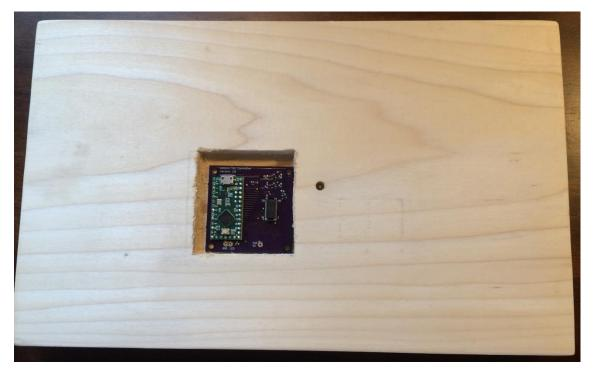
You'll have to drill a hole into the cavity for the USB cable (not done yet in this picture). The hole beside the Teensy is for a post on the keyboard. The backside picture shows the rubber feet and a hole for a screw into the post.
