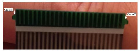
If the FPC traces don't line up with the connector pins, use an X-ACTO knife to trim along the side of the cable as shown.
