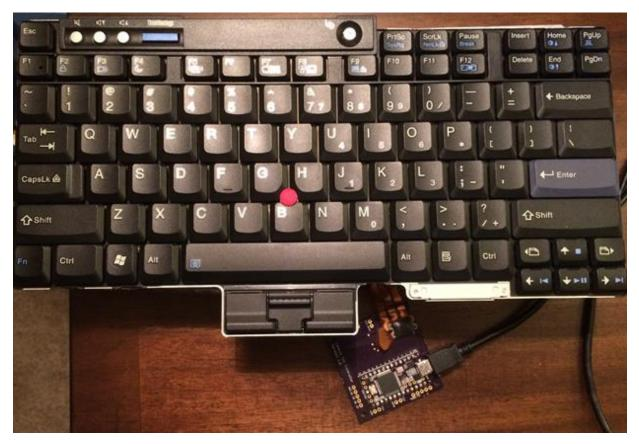
The keyboard and Teensy 3.2 USB controller card is shown below.
