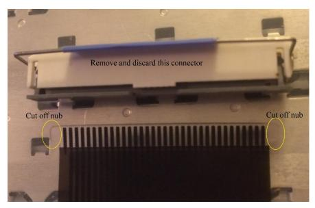
The final mod was to remove the extra thick plastic backing on the end of the cable and replace it with 2 pieces of a paper to bring the thickness back to normal for a generic FPC connector.
