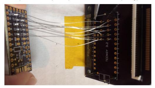
Finish the assembly by soldering 30 gauge solid wire to the remaining I/O signals marked with a small line. The bare and assembled 3.2 board is shown below.
