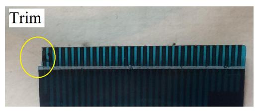
The Dell Latitude D630 keyboard needed the most modifications. It had a solder-less connector on the end of the FPC cable that was easily removed. Then I trimmed off the side nubs and made a notch to align the contacts.
