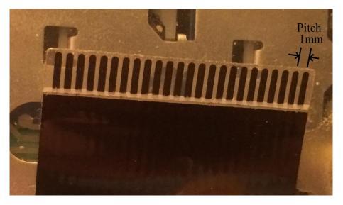
The picture below shows a standard 24 pin FPC Cable with a 1mm trace pitch.
